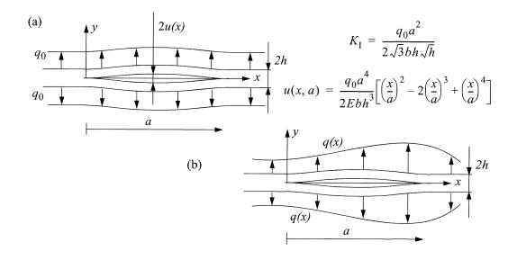
3. A beam of width b has a crack according to the figure below and is loaded in pure bending. Determine the stress-intensity factor when  $h \gg 2a$ . The material is linearly elastic.
