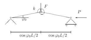
3. Determine the equilibrium paths of the simple structure shown, consisting of rigid bars and elastic springs. Investigate also the stability of the equilibrium paths. Investigate especially cases  $k_1 = k_2$  and  $k_1 = 5k_2$ . What kind of real structures these models imitate?
