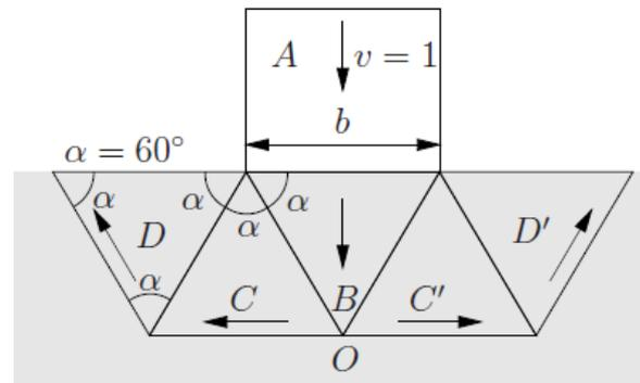
$$F \cdot v = 2\{v_{BC}l_{BC} + v_{CO}l_{CO} + v_{CD}l_{CD} + v_{DO}l_{DO}\}k,$$
