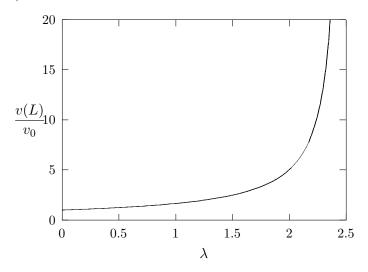
Notice that the displacements start to increase rapidly when  $\lambda > 2$ , which is about 20 % of the critical buckling load  $\lambda_{\rm cr} = \frac{1}{4}\pi^2 \approx 2.467$ . The superposition principle is not valid for the axial load P. Why?
