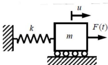
Express the harmonic excitation by Fourier series and determinate the response of the undamped 1DOF vibrator. Draw curves for the excitation approximation and the response using one and three terms of Fourier series.
