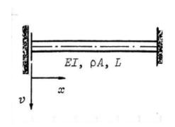
1. Determinate the stiffness matrix using two beam elements. Condense statically the rotational DOF. Determinate the lowest eigenpair by the inverse vector iteration. Use the lumped mass approximation. By Sturm's sequence rule find out whether the second eigenfrequency is higher than  $\omega = 35\sqrt{EI/\rho AL^4}$ .
