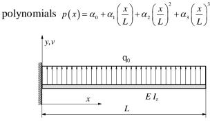
2. Solve the estimate of deflection curve v(x) for the beam (*E I*<sub>z</sub>) below. Use the principle of minimum potential energy. Model only symmetric half of the beam and choose kinematically admissible trial function from polynomials
