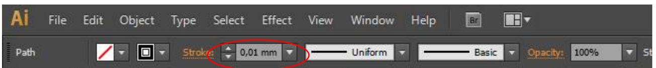
Fig. 7 adjusting the line thickness.
