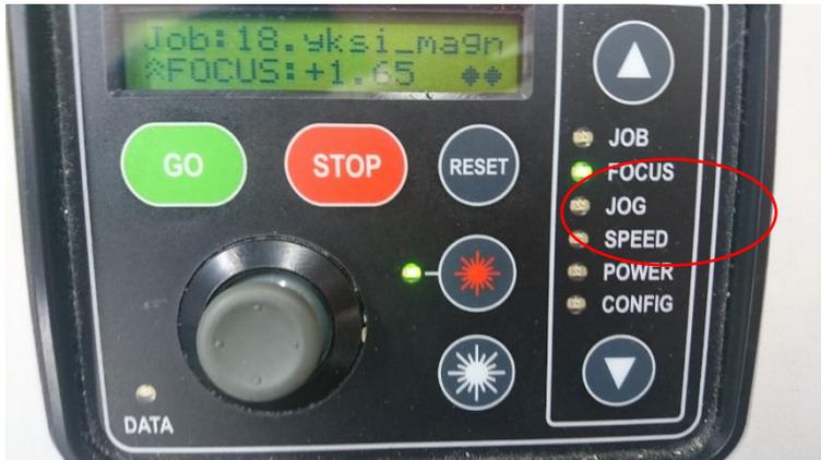
*Fig 1: Control panel in focus mode*
