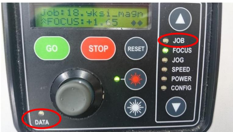
*Fig 11 Choose Job from control panel and make sure that the Data light has stopped flashing.*
