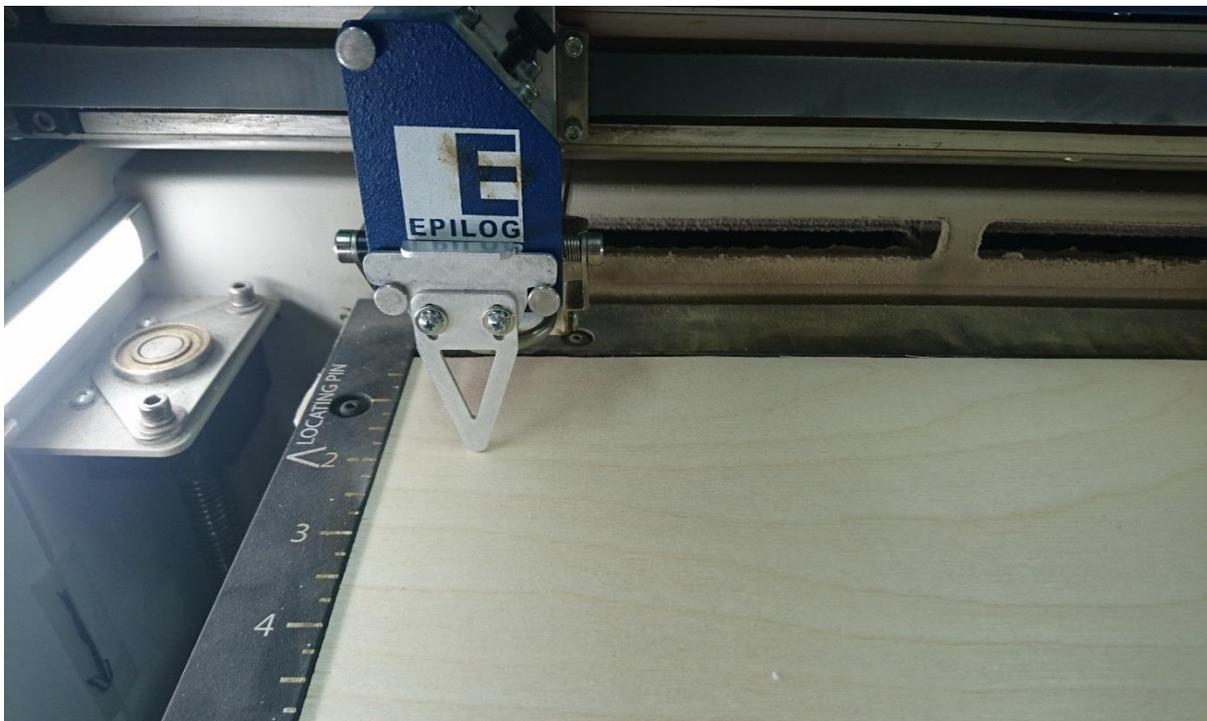
*Fig 2: Focusing triangle at right height for 6 mm plywood*
