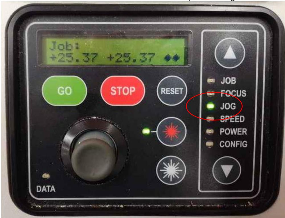
Fig 3: Control panel in JOG mode
